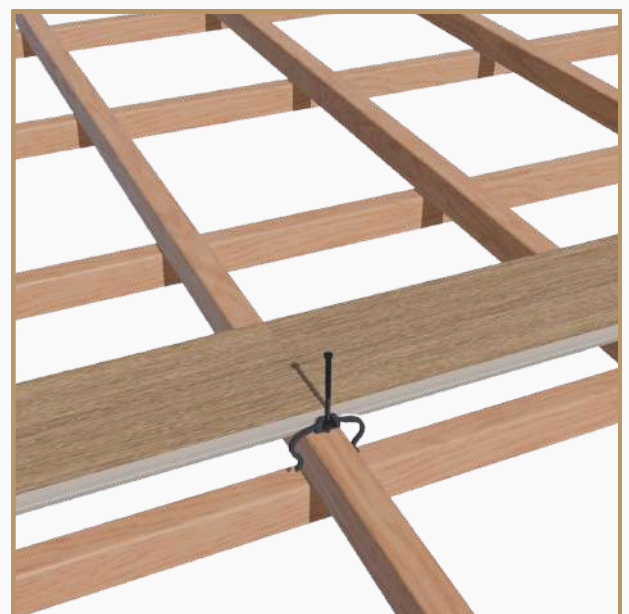
DOUBLE JOIST FRAME
